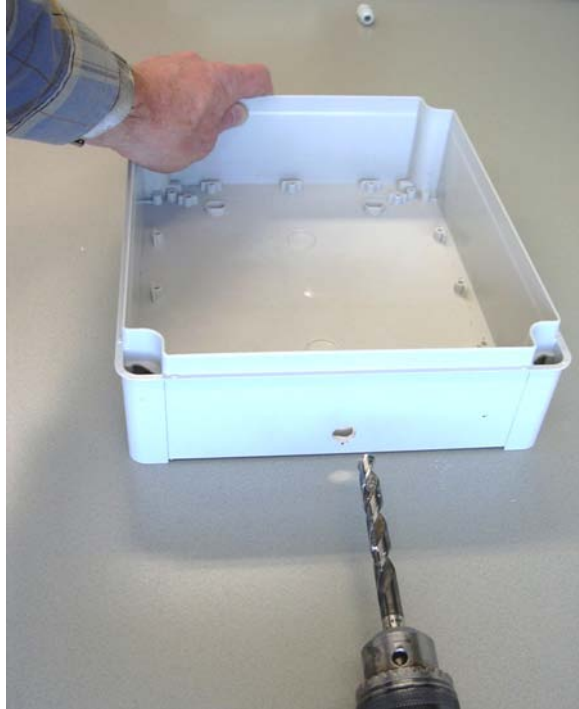
Figure 3. Drilling the hole (12 mm)
