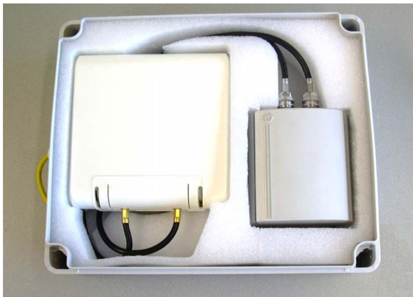
Figure 26. 4080 IP-DECT and directional antenna in their positions.
