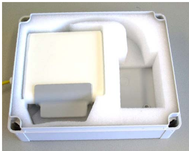
Figure 10. 4080 IP-DECT in its position in the cabinet.
