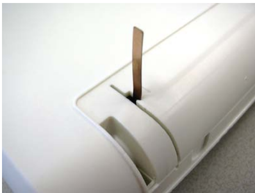
Figure 7. Detail of antenna in lock.
