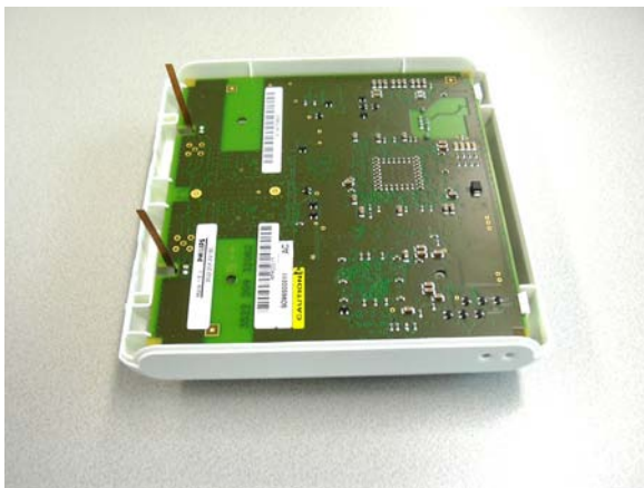
Figure 5. Bend Antennas carefully into vertical position.
