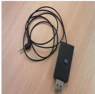
Hardware update kit comprises an USB connector and an audio jack connector.
