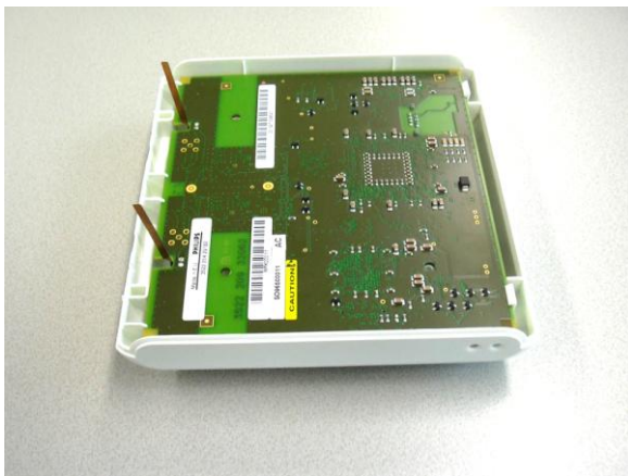
Figure 5. Bend Antennas carefully into vertical position.
