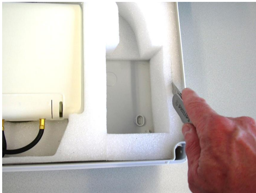
Figure 25. Cutting the foam to allow the antenna box to fit into it, in the required position.
