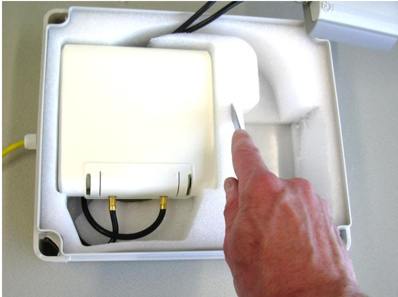
Figure 26. Cutting the foam to allow the antenna box to fit into it, in the required position.
