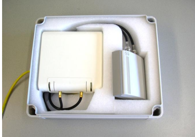
Figure 24. Antenna box does not fit into the hole.
