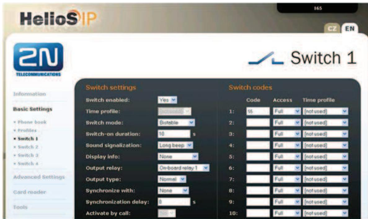
The screenshot shows the HelioSIP configuration interface for 'Switch 1'. The page is divided into two main sections: 'Switch settings' and 'Switch codes'.
