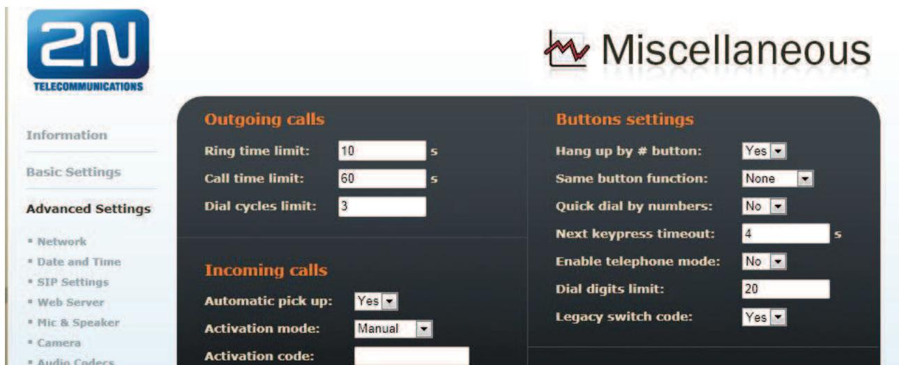
The screenshot shows the HelioSIP configuration interface for 'Miscellaneous' settings. The page is divided into two main sections: 'Outgoing calls' and 'Buttons settings'.
