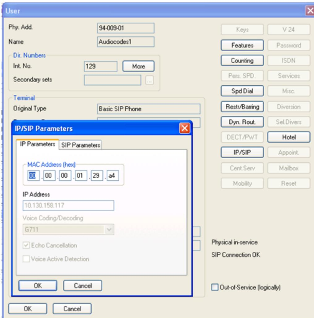
3) For other tests configure the user (extension number) to Open SIP phone as below.
