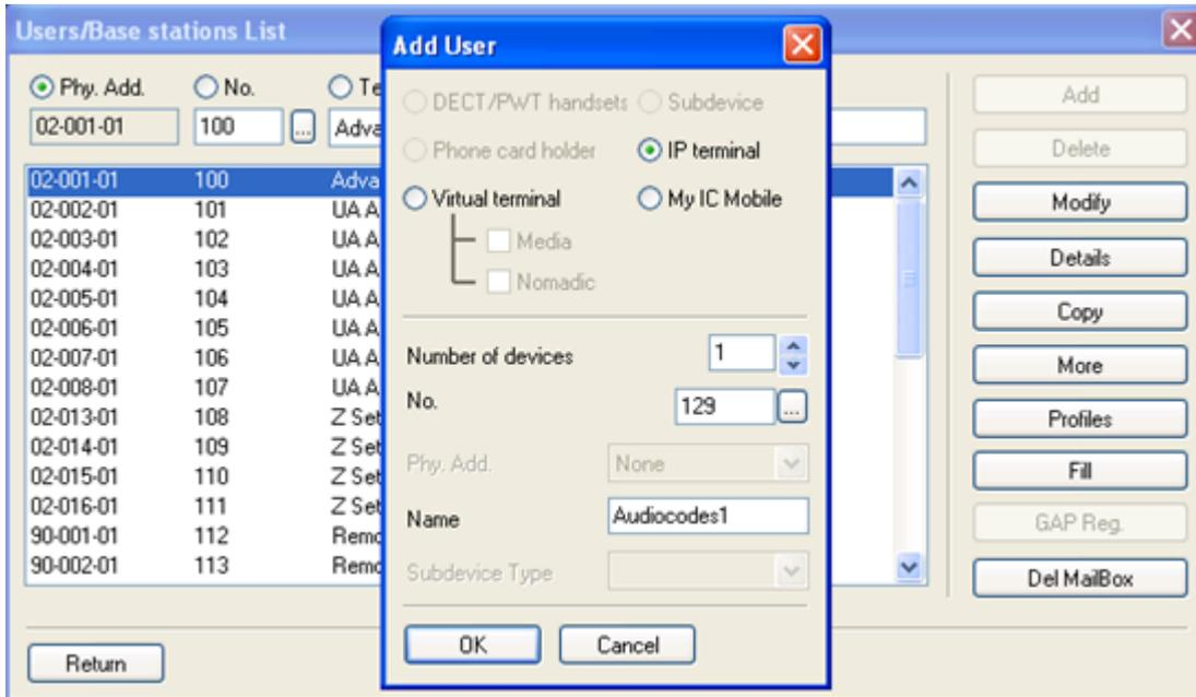
2) After creation of the user modify the (extension number) IP enabler to Basic sip phone from for the fax calls.
